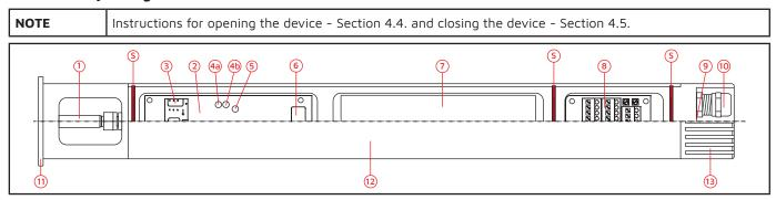
Remove the plug of the battery connecting cable from the socket (6). The plug of the connecting cable to the battery can only be removed after pressing the locking lever on the plug socket.
