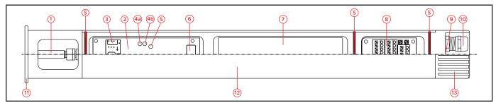
Release lock screw (13) counterclockwise and pull off together with housing tube (12).
