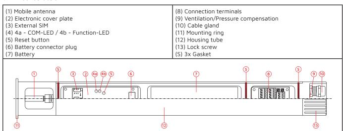
The mobile radio antenna (1) can be unscrewed and replaced with another one, e.g. a level pipe cap or directional radio antenna.
